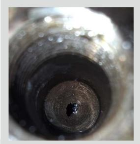
**Shown here** is a small hole in the oil filter housing where the port should have been bored completely through. The resulting restriction in oil flow led to multiple screw compressor failures.
