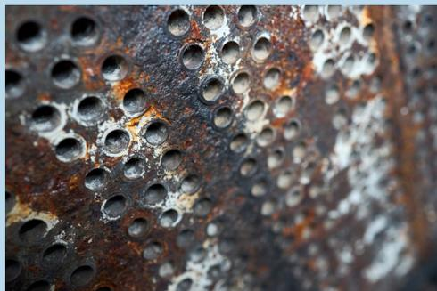
MSC received a call from a building owner who had concerns about a re-heat hot water system. The system, which was set to maintain 160°F with a steam-to-hot water heat exchanger, was slowly losing temperature over time. When the controls checked out OK, our service tech opened up the heat exchanger and found significant calcium buildup. After a thorough cleaning, we recommended water hardness testing and treatment to avoid future problems.
