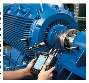
Now, with new technological breakthroughs, vibration recording equipment is capable of accurately detecting extremely miniscule movements, down to vibrations caused by a ball surface contacting a spall crater less than one-tenth the
