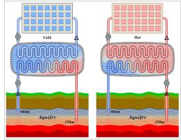
The way ATES works is fairly simple. Cool water is pumped from the ground during summer months and building heat is transferred to the water via a heat exchanger to meet cooling demands. The now-heated water is then pumped back into the ground for storage until winter when the still-warm water is brought back up and used to provide building heating. This cooled water is returned to the ground and the process continues indefinitely.
