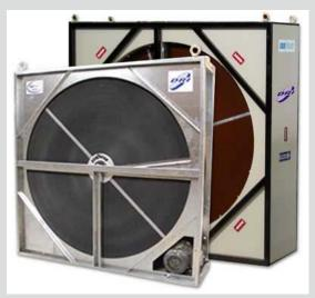
Heat Recovery - The two most common heat recovery systems are circulating glycol and heat recovery wheels. In this photo is a heat recovery wheel that rotates between the supply and exhaust duct work. A computer monitors the wheel performance and speed. This wheel is cooling 95F outside air to 79F. Pretty impressive.
