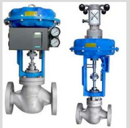
Now available on the market is a wireless steam control valve (photo by Forbes Marshall) that gets its power for the valve actuator from a thermopile arrangement strapped to the hot steam pipe, making it completely self-sufficient. The Seebeck Effect, in which two dissimilar metals will produce a voltage when there is a temperature difference between the metals, is responsible for the behavior of the thermocouples in the thermopile.
