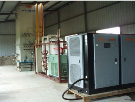
**Liquid nitrogen cooling** – The temperature of the liquefied form of nitrogen is approximately -330F, making it ideal for processes such as chemical reactors and low-temp storage. Liquid nitrogen is run through a heat exchanger and can produce temperatures of -70F and lower (normal mechanical process cooling is usually 5C). In the photo above, a low-temperature process nitrogen skid is used to cool a chemical reactor.
